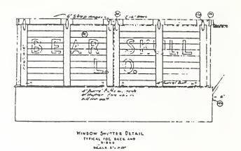
Figure 58. Lookout house window shutter detail, Plan L-4, 1931 (1932 revision), Northern District No. 1. This view is particularly interesting in that it shows how the name of the lookout might be displayed on the shutters.
